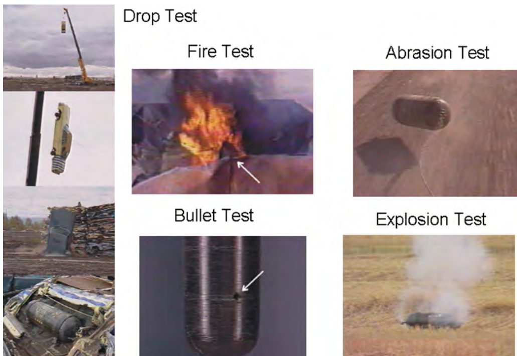
Figure 14. High-Pressure Storage Vessel Qualification Tests
