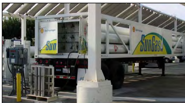
Figure 19. Hydrogen Tube Trailer
