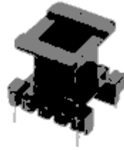
Ho Sung International. EI-2820 nylon bobbin. Core is 10 mm x 13 mm x 10 mm high. Top is 18.5 mm x 21.5 mm. Base is 22 mm x 26 mm. Four leads, 15 mm and 20 mm spacing
